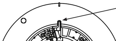
Figure 6: Removing Detector Head from Base
