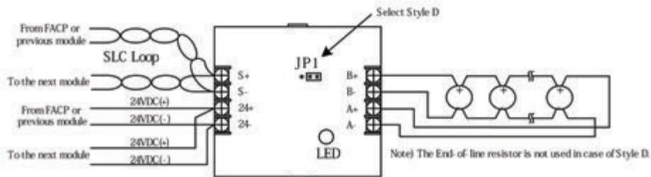
Figure 3: Wiring diagram of CIZM-4 in case of Class A (Style D)
