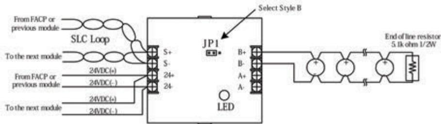
Figure 2: Wiring diagram of CIZM-4 in case of Class B (Style B)
